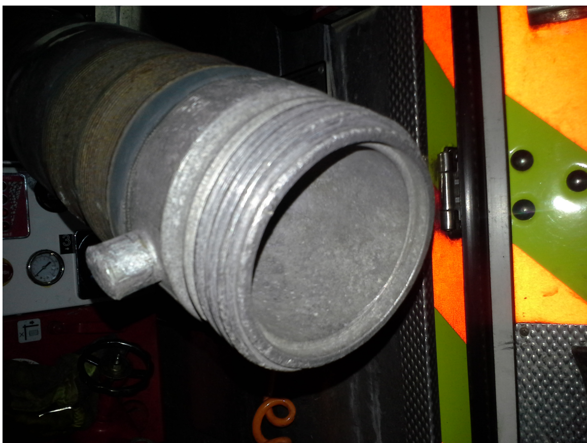
Photo 2 - 100mm Male connection on hard suction hose
