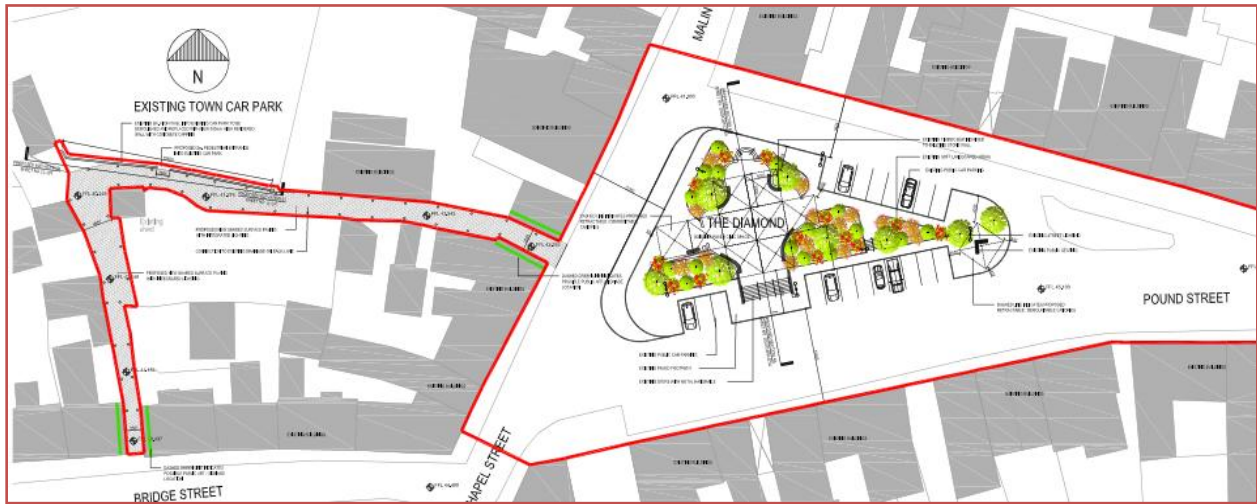
Fig.10 – A site layout plan showing the relationship between the Diamond Civic Space, Back Lane and the Existing Town Car Park, together with detail of the public realm improvements proposed to same.
