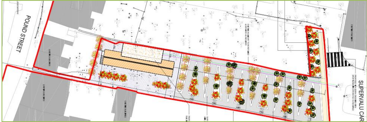
Fig.5 – A site layout plan detailing the proposed pedestrian link and urban park connecting the existing Supervalu Retail Complex with Pound Street in the context of the new Creative Hub.
