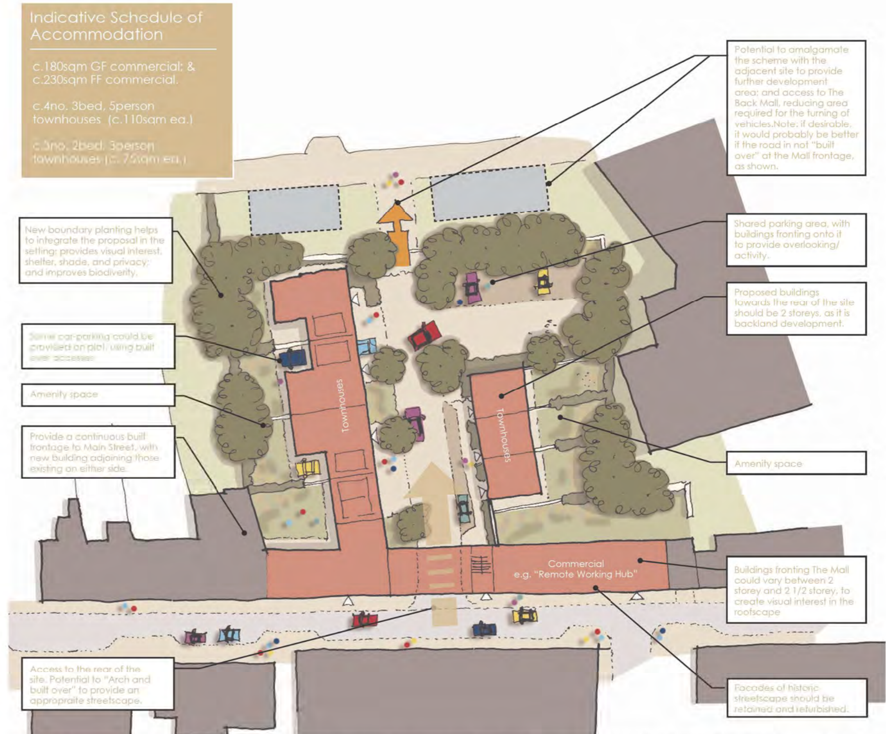
The "Ballyshannon Bakery" site - A conceptual General Arrangement showing one potential option (Mixed-use - Commercial and residential). Alternative uses/layouts may also be appropriate (scale 1:500)
