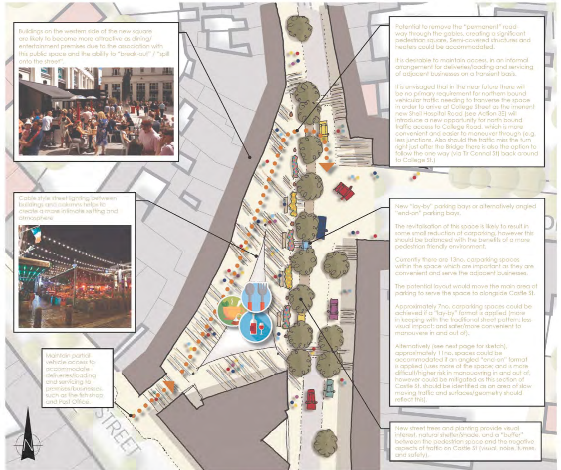
The "Gables" - A conceptual General Arrangement showing one potential option. Alternative layouts may also be appropriate (scale 1:500)
